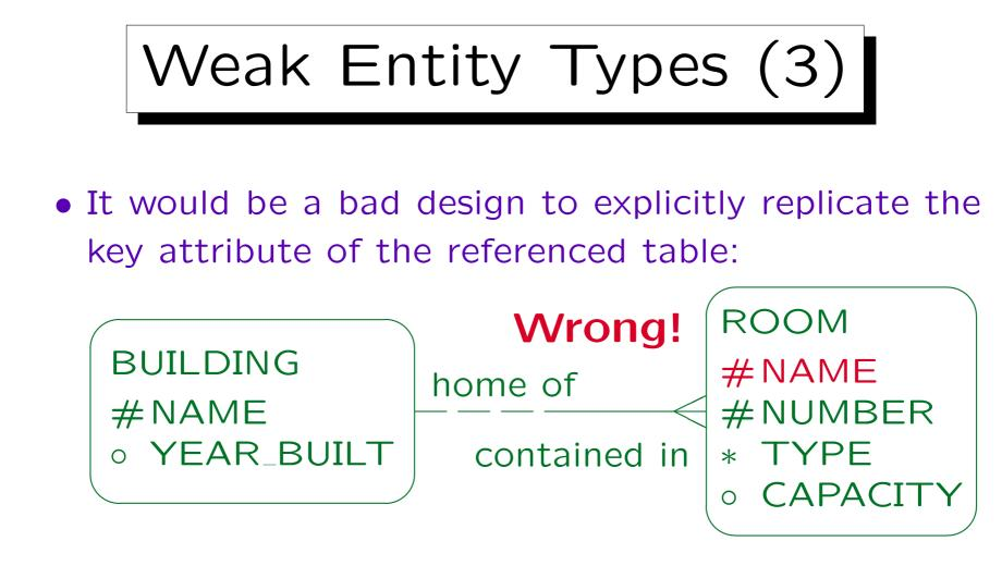
Now the constraint is needed that a room with name X is always related to a building with name X, so that the relationship is actually redundant.
