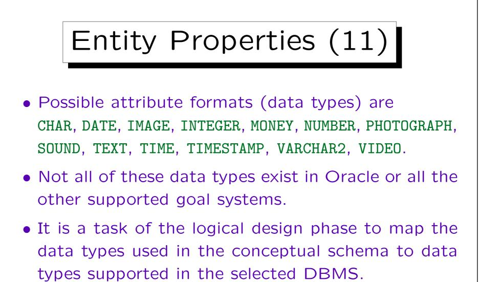
E.g. IMAGE, VIDEO, and SOUND would be mapped to a binary large object in Oracle (BLOB). The database design transformer contains mappings for various systems.
