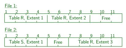
Tables R and S are stored in a tablespace which consists of two data files. Table R has three extents: Block 1 to 4 in File 1, Block 5 to 8 in File 1, and Block 7 to 11 in File 2. Oracle does not merge contiguous extents of a table. Table S consists of a single extent (Block 1 to 4 in File 2).
