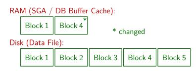
• Accesses to RAM are much faster than accesses to disk, but the RAM is usually smaller (and volatile).
