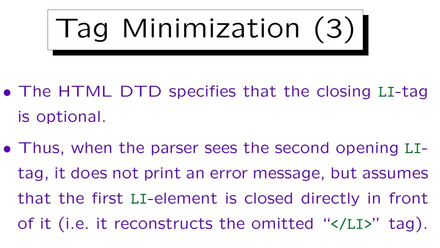
• In the same way, P-elements (paragraph) cannot be directly nested in HTML, and only the start tag is required (the closing tag is declared as optional).
