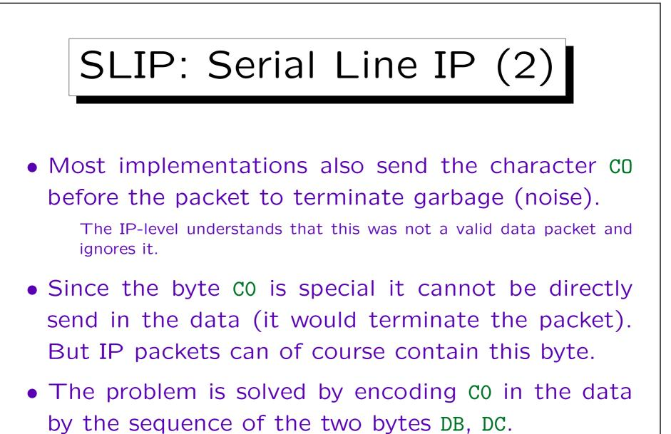
• Now DB is also special. It is encoded as DB, DD.
