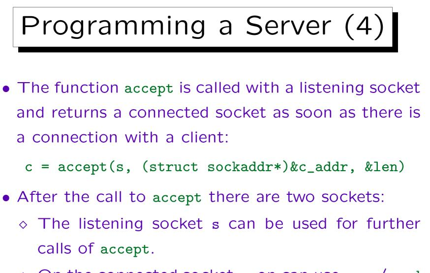
On the connected socket c, on can use recv/send to serve the client.
