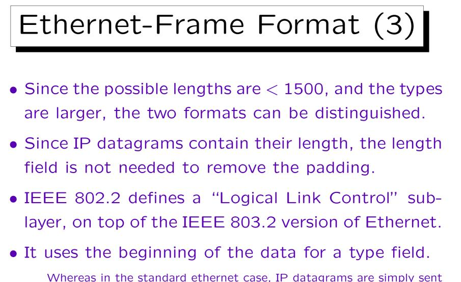
Whereas in the standard ethernet case, IP datagrams are simply sent in the data field (see RFC 894), the IEEE 802.2/803.2 encapsulation is a bit more complicated (RFC 1042).
